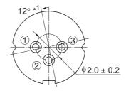
Note: 1. The beam has 12 deg offset against the package reference plane. Please take account it mounted on a board.
